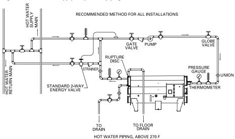
HOT WATER PIPING, ABOVE 270 F CONSTANT FLOW THRU GENERATOR
